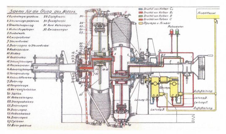
Oberurseler 160PS Umlaufmotor U III – lubrication scheme with inlet valve arrangement
