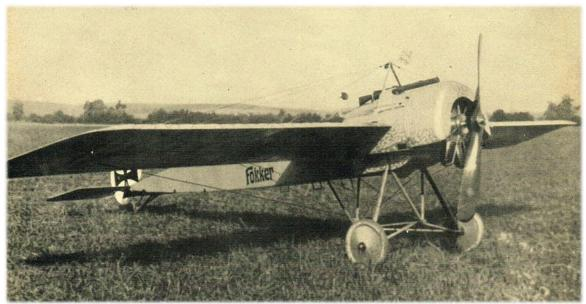
The very first German Fighter-aircraft, a Fokker E I, powered by a80 HP Oberursel rotary engine U 0
